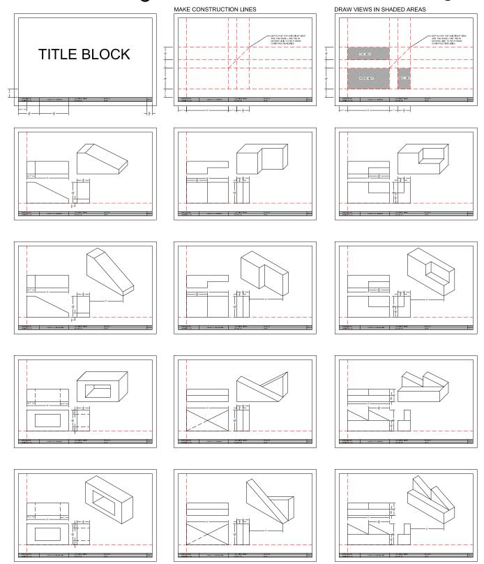
USE DRAFTING TOOLS TO COMPLETE THE VIEWS FROM THE HANDOUT AND CREATE A MULTI-VIEW DRAWING ON TYPE B PAPER ( 11 X 17). INCLUDE A PICTORIAL - OBLIQUE OR ISOMETRIC.
